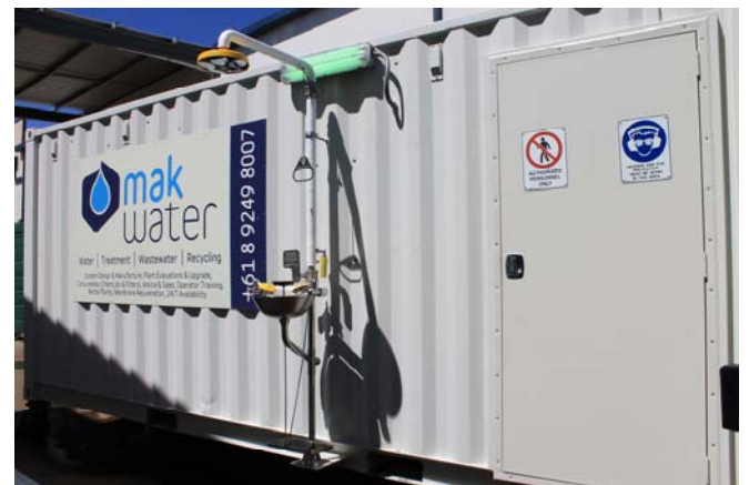
The modular brackish water reverse osmosis plant ready for delivery to the Cosmo Newberry remote Aboriginal community
